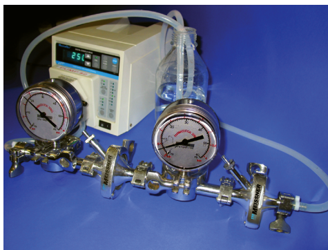
Figure 2: Bacterial challenge test apparatus showing differential pressure between two inline 47-mm diameter filter disk holders in series, with the challenge filter upstream and the analysis filter downstream, connected by sanitary piping to a peristaltic pump which recirculates the challenge microorganism.
