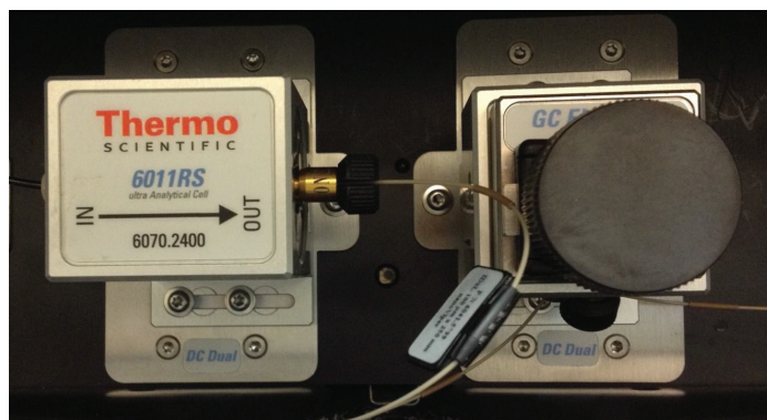
FIGURE 3. Electrode Arrangement for Redox Cycling of Catechol Compounds.
